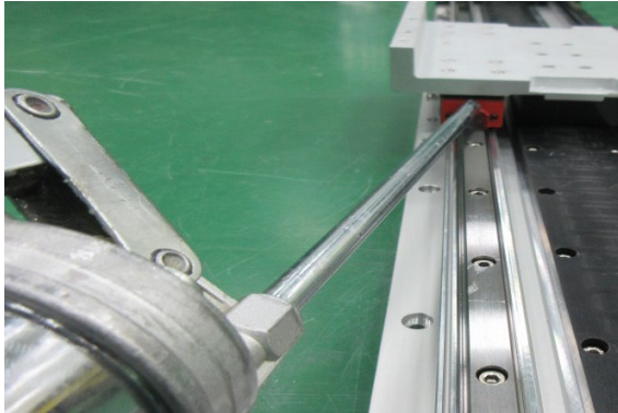
Fig. 7.7: SSA 13, 18, 20 grease maintenance kit
