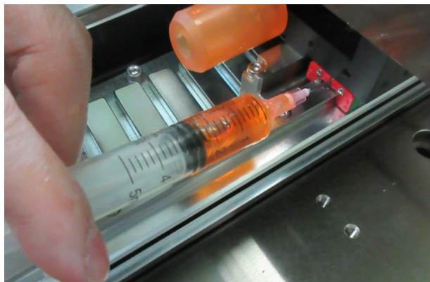
Fig. 7.6: SSA 08, 10, MGN Block grease maintenance kit
